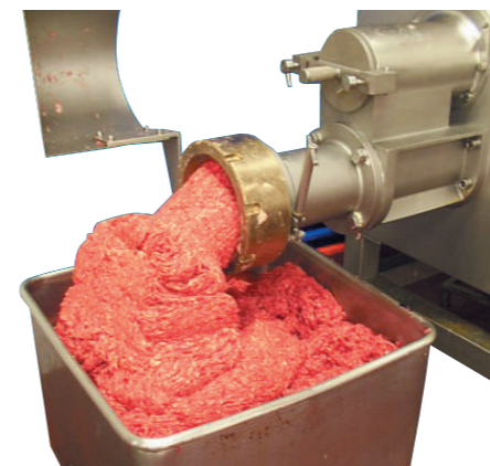
Beef Trim. 2nd Mince - 3600 kg / hr (60kg/min). Processed with 6400 66 Mixer Mincer through a 3 mm Hole Plate.
